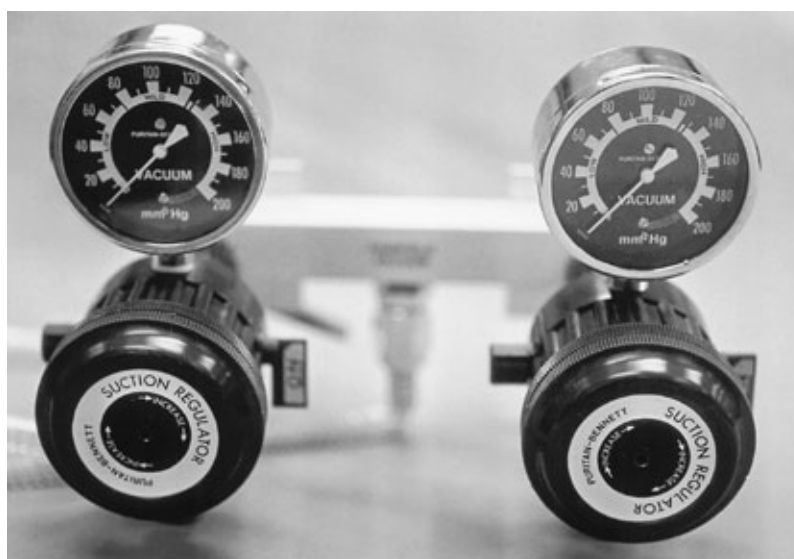
FIGURE 6-18 A Puritan-Bennett suction regulator with vacuum pressures ranging from 0 to 200 mm Hg.
